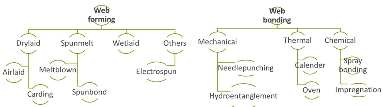
Figure 1 Web forming and web bonding processes
